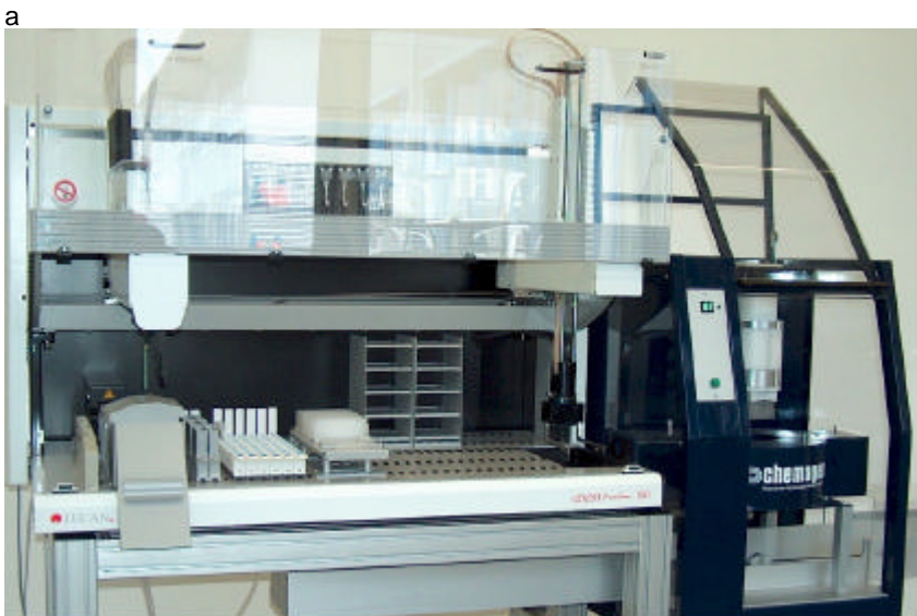
Fig. 1: Tecan Freedom 150 Workstation with chemagic Magnetic Separation Module I attached. Robotic arm can load the carrier axis through the worktable.
